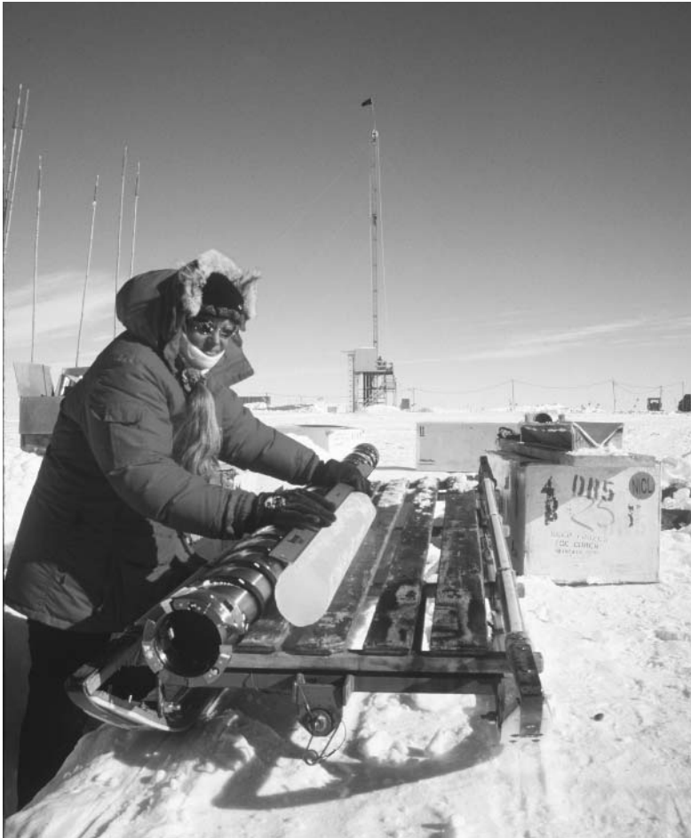
Fig. 2.6 Removing ice from a core just recovered from 90 m deep at Siple Dome, Antarctica. The drill is on the sled beside the core. In the background is the support tower for a larger drill that can recover cores to a depth of 1,000 m (From Taylor K 1999. Rapid climate change. American Scientist 87 : 320–327).
